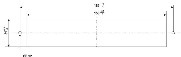
**9.2 VÝŘEZ V PANELU PRO XH260V**
